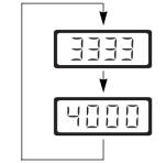
② If you want to change the sewing speed, press the E/Prg button. After seeing the speed programming screen, press buttons A and B to program the speed you want.
