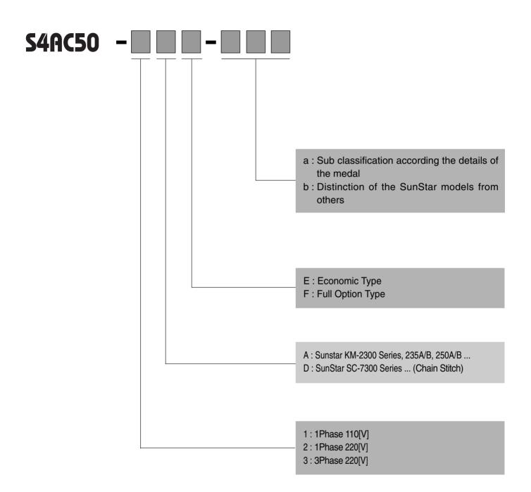
OREDER Ex. S4AC50-2AF refers to SERIES4, 1Phase 220V, FULL FUNCTION CONTROL BOX for normal drop feed.
