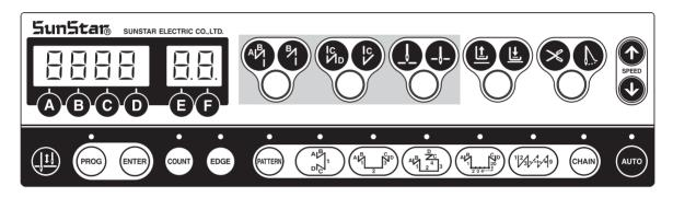
Method of initializing: Turn the power on by simultaneously pressing the buttons in the figure above which are the start B/T button + end B/T button + needle plate up/down stop button.
